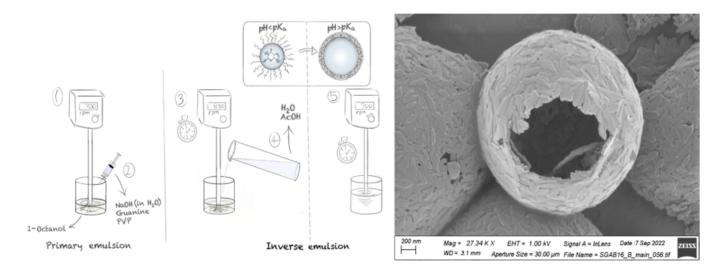
Left: Scheme showing the stages of the crystallization process;
